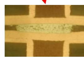
Board to board connection by conductive paste
