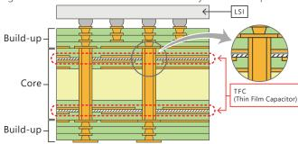
GigaModule-4EC: TFC embedded in build-up layer of coreless PCB
